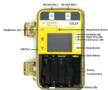
Figure 2: Anabat Swift acoustic monitor internal components
