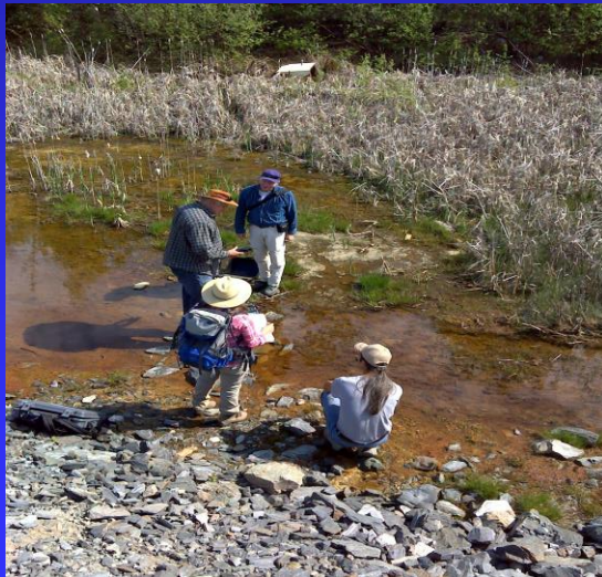
Very high conductivity readings likely indicate high levels of arsenic and other mine leachates
