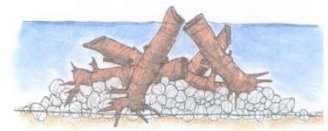
D4 SUBMERGED LOG TANGLES & STONE PILES N.T.S.
